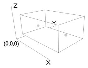
• Angles are specified in vertical polar co-ordinates, with azimuth being a direction in the room horizontal plane between -180 and +180 degrees, with 0 degrees being straight ahead down the y-axis, while elevation being a tilt to the room horizontal plane between -90 (down) and +90 (up).
