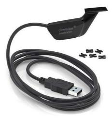
The HT-1 head tracker is a USB device that sends real-time orientation data of the head tracker pod. The head tracker pod can be attached to the listener's headphones to input the pitch (elevation) and yaw (azimuth) movements of the listener's head into the generator.
