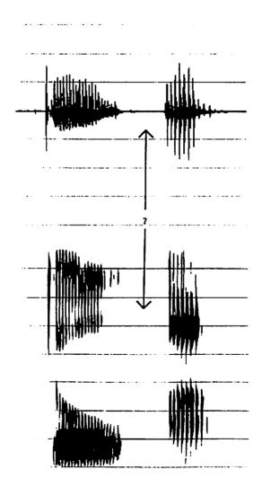
Figure 4. Speech waveform and wide band spectrogram of daughter with intervocalic tap, adult male speaker. Divisions of vertical axis: 500 Hz. Time axis: 500 ms.
