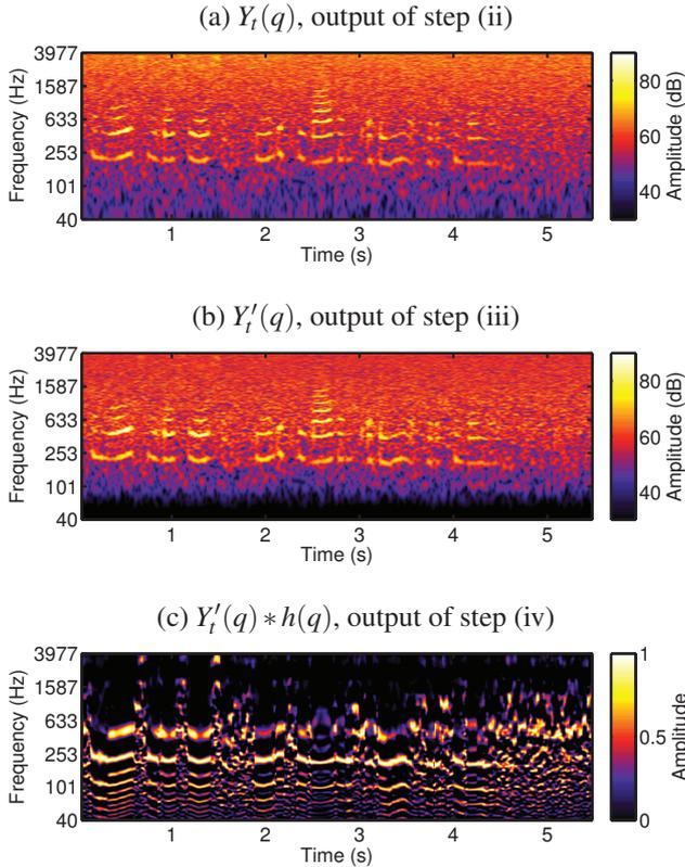
Figure 3: Output of various steps of PEFAC for a speech file corrupted with white noise at  $-5$  dB SNR. (a) Noisy speech log-frequency spectrogram, (b) compressed noisy speech spectrogram, and (c) output of the pitch analysis filter normalized at each frame to its peak value.
