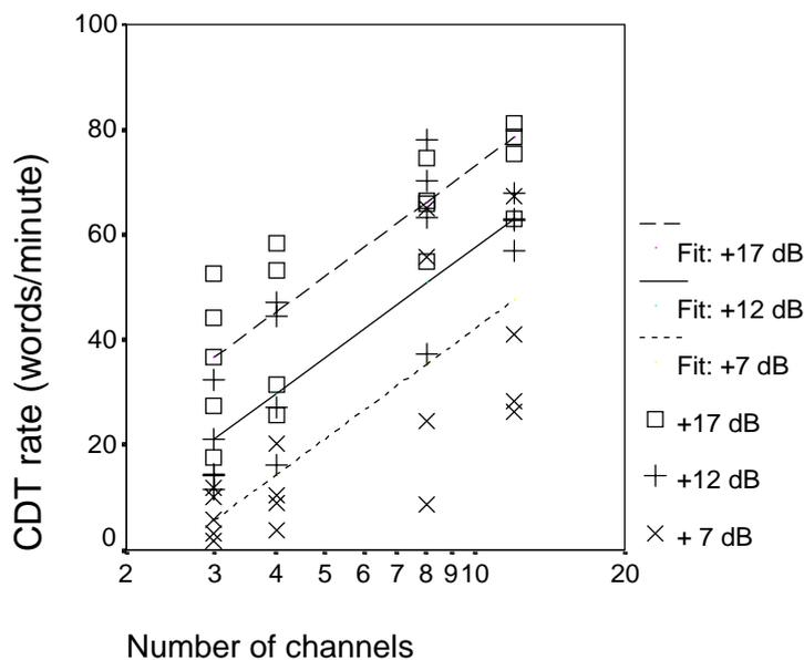
Figure 4: Regression of SNR and  $\log_{10}$  (number of channels) onto CDT rate for processed speech excluding scores in quiet. The lines are calculated from the regression equation:  $rate = -49.19 + (SNR\ dB) \times 3.091 + \log_{10}(number\ of\ channels) \times 69.61$ . Individual symbols are mean CDT rates for the 4 individual subjects at each SNR. The regression accounts for 65.9% of the variance.<sup>iii</sup>
