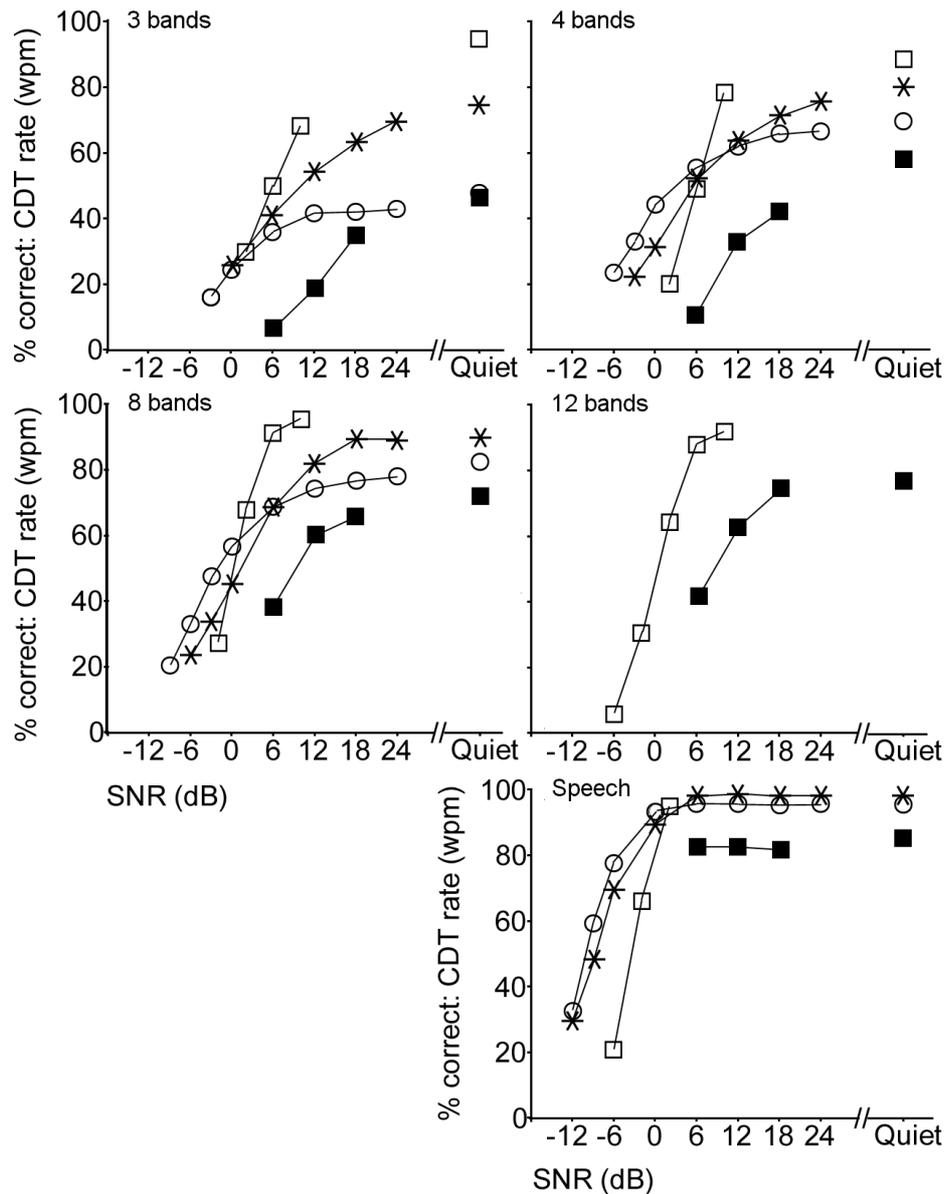
Figure 6: Effect of SNR on CDT, HINT sentence, vowel and consonant identification. Each panel shows data with a different number of channels. Symbols: • CDT rate; • Words correct in HINT sentences; • Vowels correct; \* Consonants correct.
