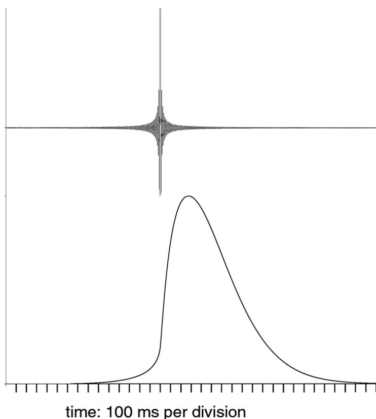
*Figure 2: Response of slow envelope extractor (lower panel) to a band-limited impulse (upper panel).*
