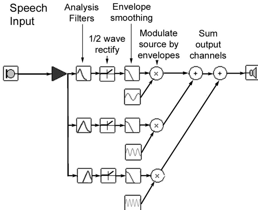
Figure 1 Block diagram of signal processing for a three-channel sine-excited vocoder
