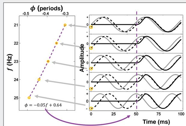
Figure 1: A diagram of a system with a group delay of 150 ms (purple dashed lines). Right Panel: Sine waves (grey) at 21 to 25 Hz are input with starting phases of 0. The output (solid black) starts 150 ms later; its Fourier Transform (dashed black) extrapolates back in time to different starting phases (yellow circles). Left panel: the transformed phase (relative to cosine) as a function of frequency. The slope of the fitted line is the negative sign of the delay in seconds.
