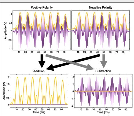
Figure 2: An example of the positive polarity (top left) and negative polarity (top right). Adding the two polarities enhances the envelope and cancels the fine structure. Subtraction cancels the envelope and enhances the fine structure.
