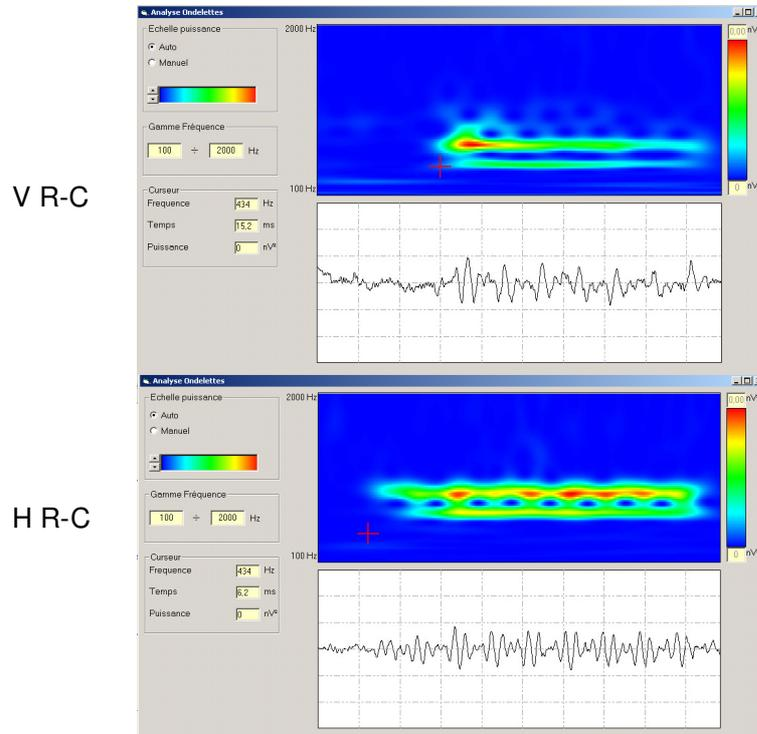
**Fig. 18:** Peripheral (H) and central (V) TFS waveforms evoked by the 85 dB SPL stimulus and their TFA. In the peripheral channel, there is no energy at the frequency of the expected CDT (cross). In the central channel, the CDT frequency does not appear earlier than the visually identified temporal signal.
