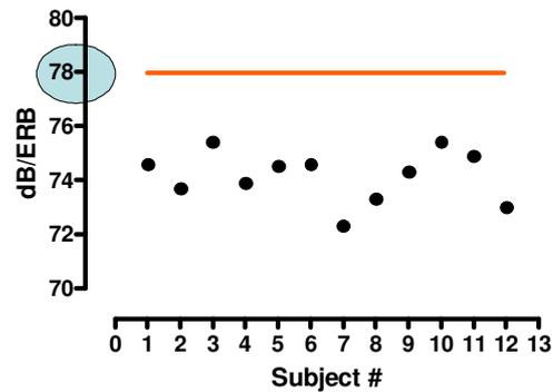
**Fig. 9:** Procedure used to define the masker level needed to mask perception of the FFR stimulus in normal hearing young listeners. It led to a TEN level of 78 dB/ERB.
