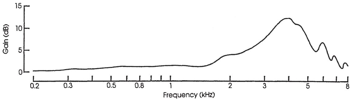
Some understanding of this response can be gained by imagining the ear canal to be a short cylindrical tube closed at one end, as shown below. The input signal is the sound at the opening of the model ear canal, the output is the sound at the closed end of the tube, with the system being the tube itself.
