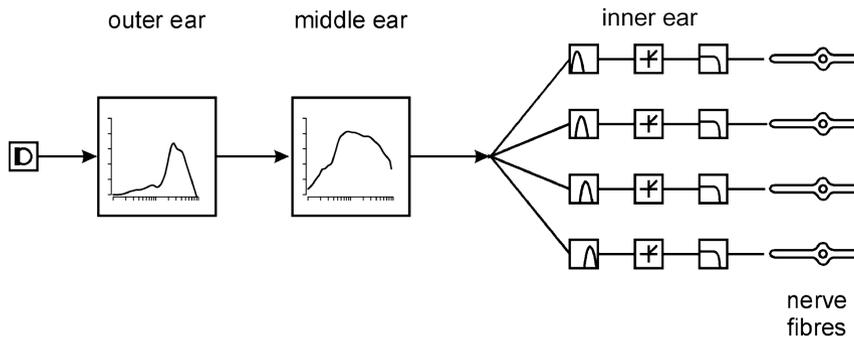
The original acoustic wave in the environment is first transduced by the microphone depicted at the left-hand side of the figure. The resulting electrical wave can then be processed by the rest of the systems in turn, resulting in the representation of the sound that is sent to the brain by the auditory nerve fibres at the far right.
