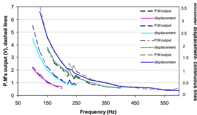
**Figure 4:** Relationship between the displacement of the vibrator and read-out voltage across the photometric device (P.M) for the rotary vibrator.
