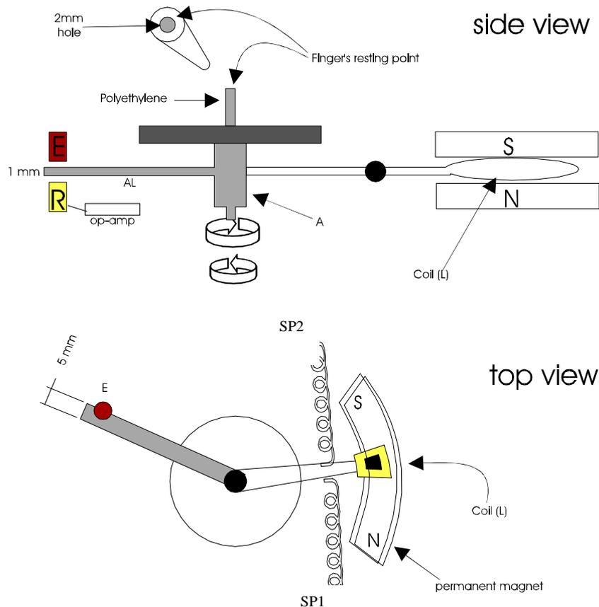
**Figure 2:** The components of a rotary vibrator (not to scale).
