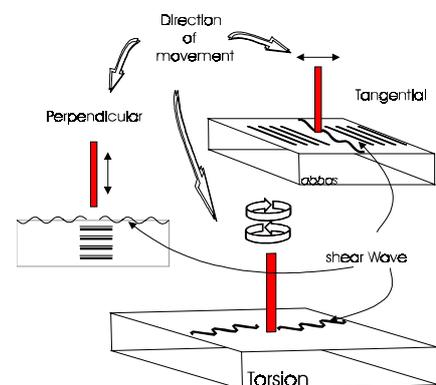
**Figure 1:** Propagation of waves generated by three methods of oscillations
