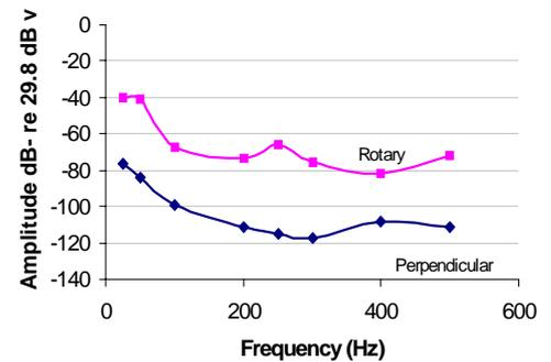
**Figure 6:** Absolute thresholds for perpendicular and rotary vibrators. The ordinate is input voltage to the vibrator in dB referred to the maximum voltage available.
