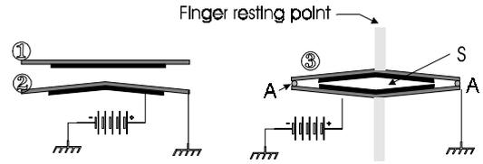
**Figure 3:** Piezo-electric benders. (1) Relaxed (2) Activated and (3) assembly of a perpendicular vibrator (not to scale).
