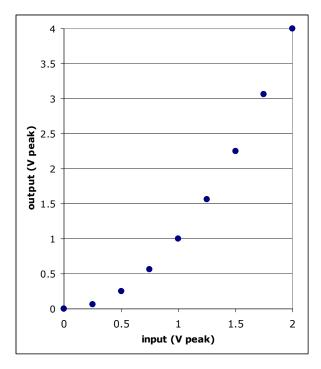
Secondly, plot the input/output function for a sinusoidal input of varying levels. You would then obtain the curve at left. Although this clearly goes through the origin (0,0), it is far from a straight line. Therefore, the system cannot be homogeneous, so cannot be LTI.
