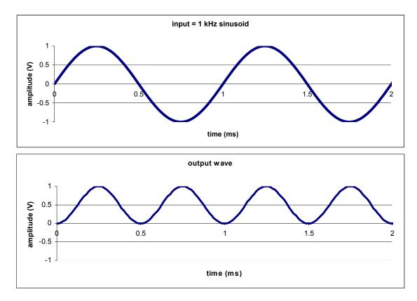
Note that the output to a 1 kHz sinusoid is still a sinusoid, but it is at a different frequency. Hence, the system cannot be LTI.
