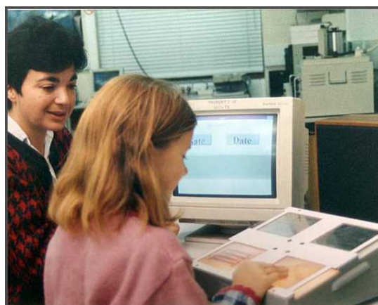
Figure 4. Interactive speech perception testing in the mid-1990s at Wolfson House (Valerie Hazan and subject), using formant synthesis and a touch sensitive response box—before the advent of touch sensitive computer screens. Two spectrographs can be glimpsed in the background, on the left Houde’s real-time and on the right the drum of a Kay mechanical scanner.
