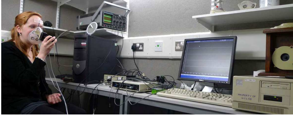
Figure 2. Inside one of the recording rooms. The experimenter is using a Rothenberg mask to gather airflow data. On the bench are a portable Laryngograph, calibration equipment for the airflow unit, and a PC adapted for multi-channel acquisition.
