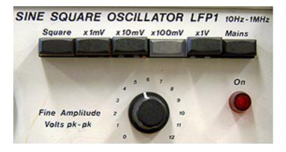
In this example the x100mV button is depressed denoting that all the values on the dial should be multiplied by 100mV. The dial is halfway between the 5 & 6 so an output voltage of about 550mV has been set. Because it is difficult to set a voltage accurately using only this dial, all output levels should be checked using a voltmeter
